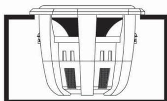
Box is given as internal air volume including driver displacement
