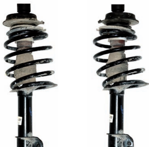
Correctly fitted top plate
