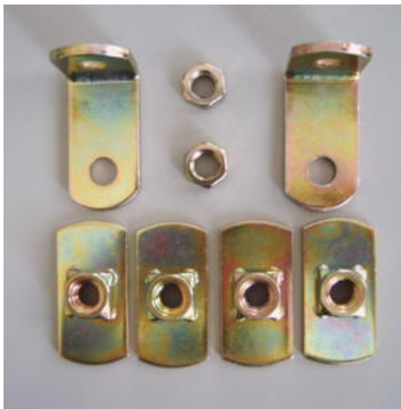
Drill Floor under rear seat at optimum position for these mountings – From http://www.fiatclassic.com
