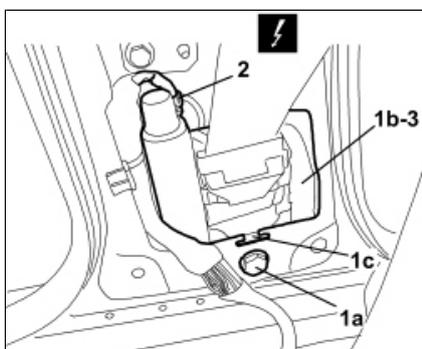
1. Undo bolt (1a) and move pretensioner (1b) by releasing retainer (1c) from its housing on the pillar.
