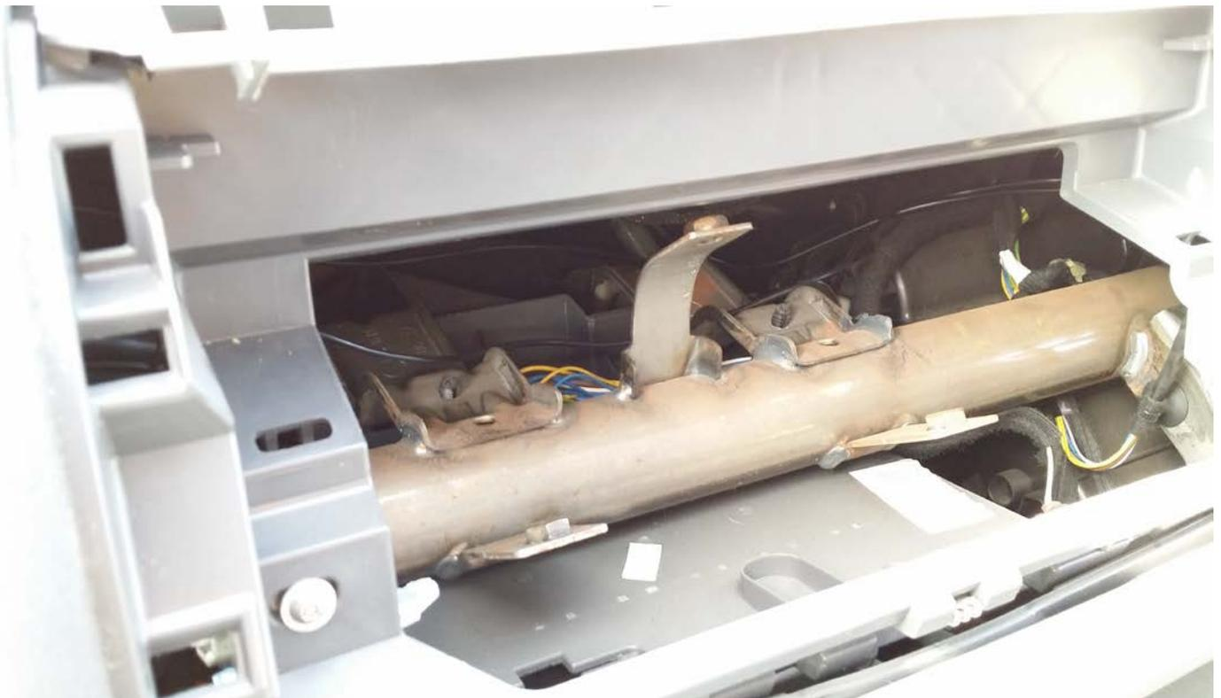
Time to move forward to the front, and the hard(er) bit. When you yank out the standard stereo you'll see a dirty great plug on the back with a lever underneath. It's hard to see properly until you release the poxy aerial cable plug (I found that hard never having seen one before, but you need to push in a little plunger underneath it to allow the ridiculously short aerial lead to be pulled out. A third hand would have been useful but a struggle and sporadic blasphemy eventually succeeded.
