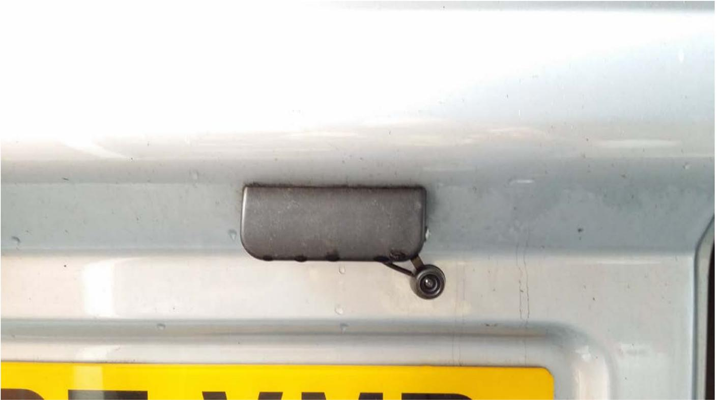
And this is how I got the cables up from the camera into the van inside the nearside back door, through the tricky rubber pipe (I used a long, bendy sink drain cleaning spring to drag the cables through):
