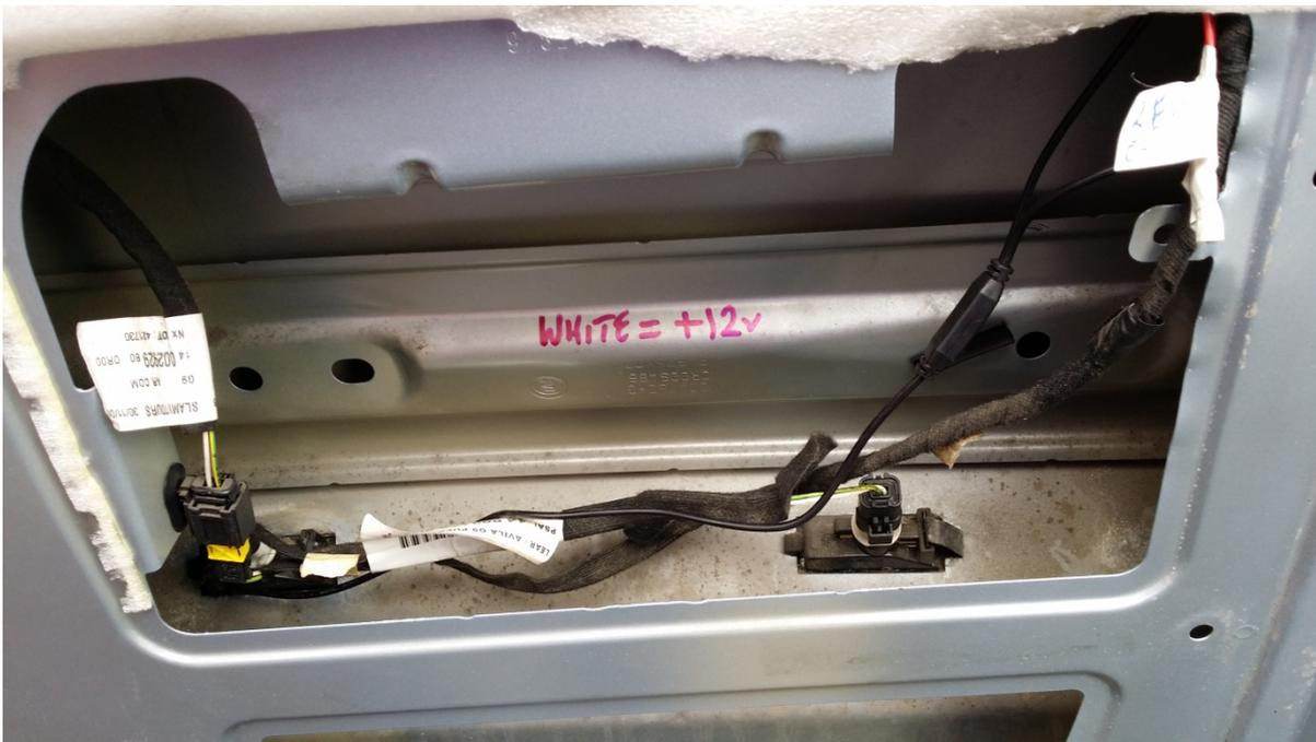
I ran the camera cables up from the floor in the passenger foot well into the gap above the glovebox (a pig to get the top plastic cover off in pic below – use the Force!):
