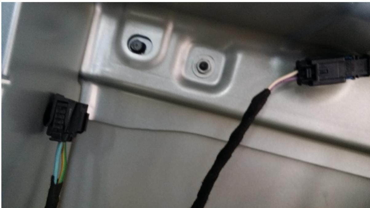
The other side of the van had no power feed cable, just the speaker pair, so I got on with mounting the speakers on the panels and that was that taken care of. On the passenger side I also found a whole bunch of cables terminated in safe connectors but just lying spare. I think they are also for caravette conversions although one very thick yellow cable may just be for the optional electric rear air conditioning unit I read about somewhere.
