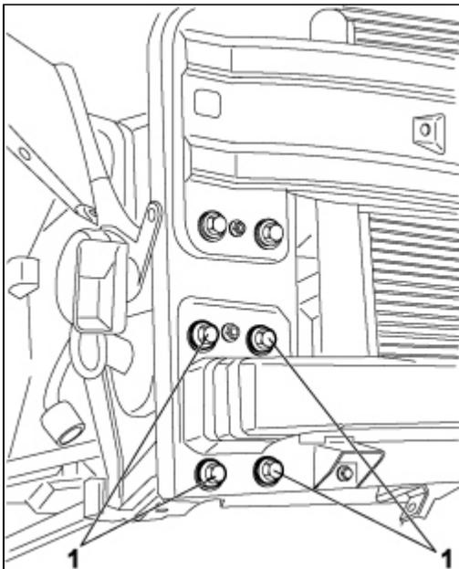
1. Undo the track control arm side panel/strut fixing bolts.
