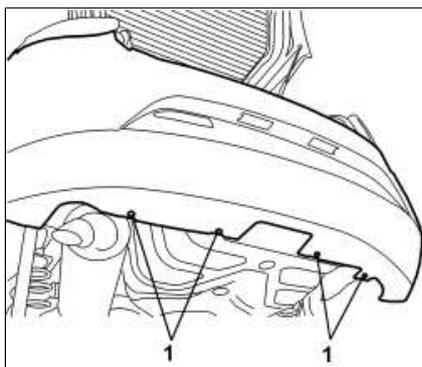
1. Undo the lower bolts fixing the bumper.
