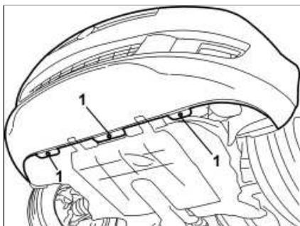
1. Undo the lower bolts fixing the bumper.
