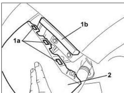
1. Release the side ends (1a) of the bumper from the retainers (1b).
