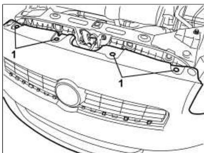
1. Undo the upper bolts fixing the bumper.
