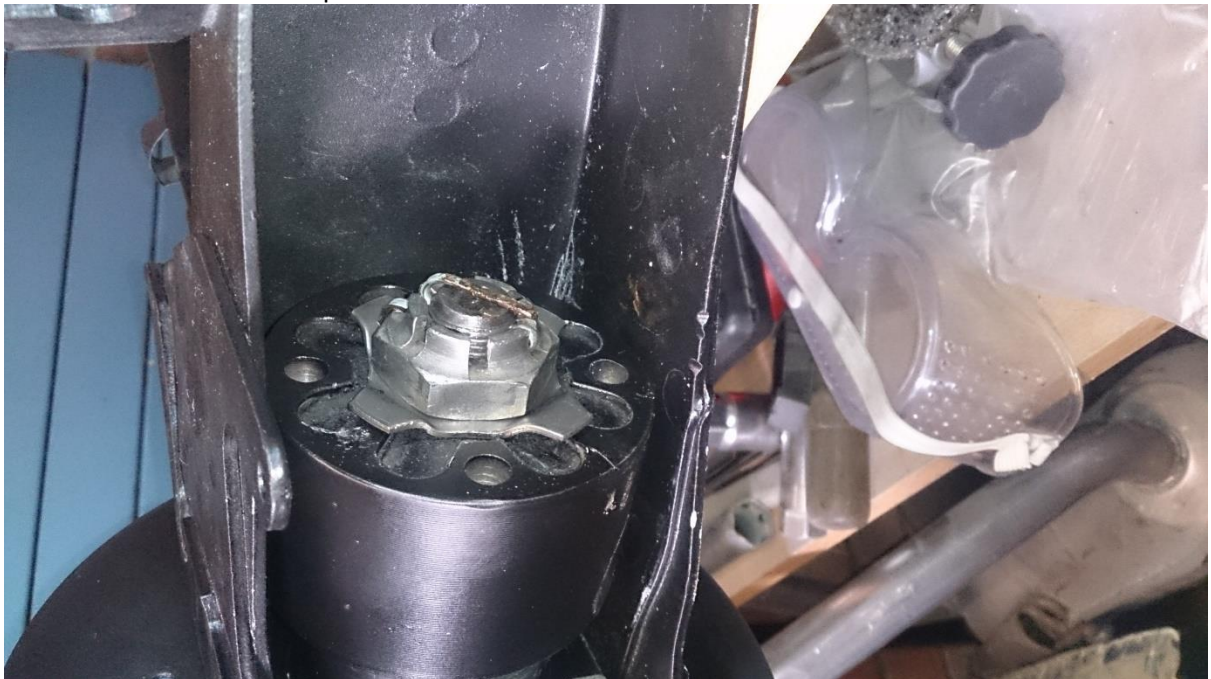
Bar used to check preload. Note centre mark and mark set at 4.3 inches from centre
