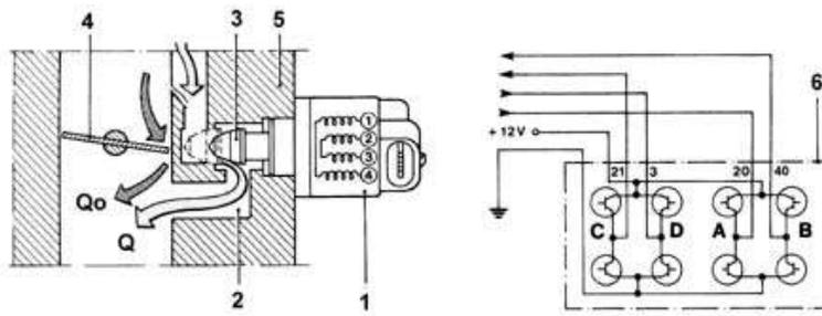
Q, Air flow rate regulated by the actuator (variable)
