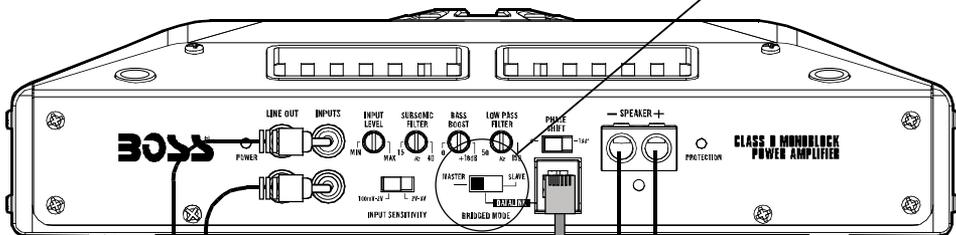
To Audio Outputs of head unit or Subwoofer outputs of a signal processor
