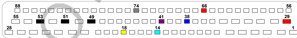
Normal or Recovery Mode Pins
