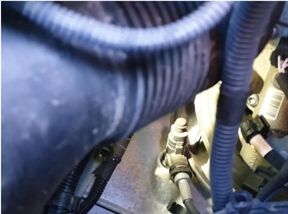
**Bleeding nipple with cover removed. Note the knurled knob for undoing the nipple.**
