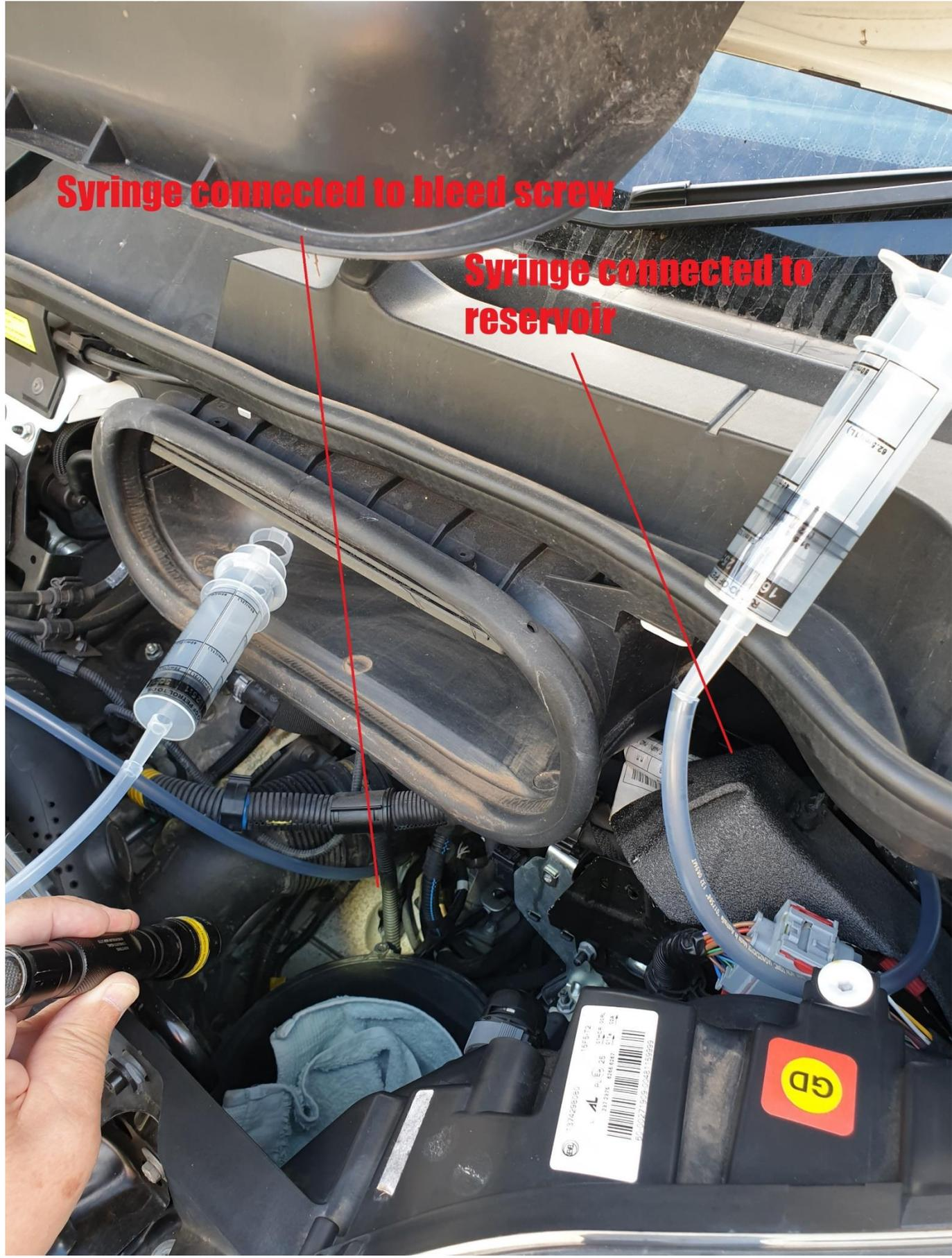
**Syringe line connected to bleed screw**
