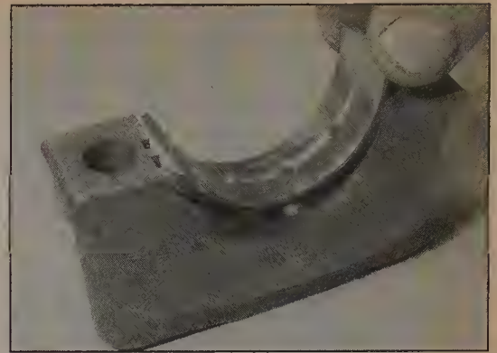
12.8 Locating a lower half main bearing shell in its cap
