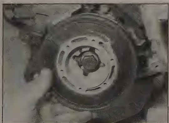
2.14b ... and remove the pulley from the front of the crankshaft
