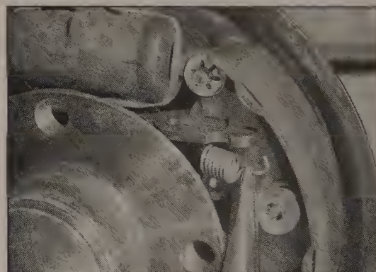
5.7a Unhook the self-adjuster mechanism from the trailing shoe ...
