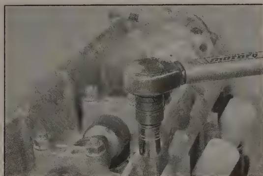
9.52b Tighten the cylinder head bolts to the Stage 1 and Stage 2 settings using a torque wrench
