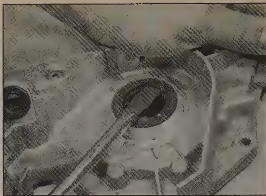
13.6 Prising the oil seal from the oil pump housing
