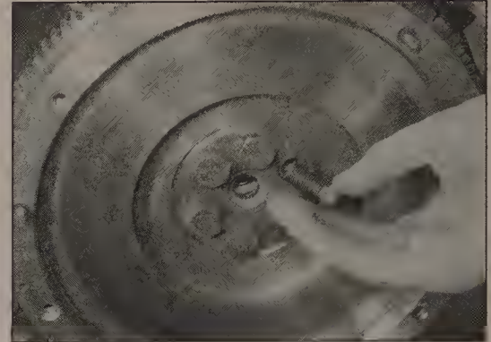
10.8b Inserting the flywheel bolts
