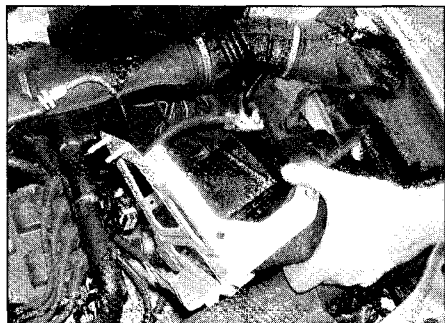
2.8 Removing the battery tray
