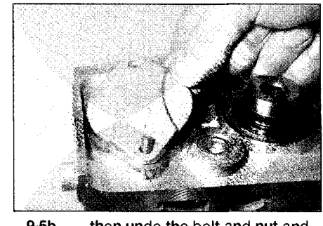
9.5b ... then undo the bolt and nut and remove the cover plate over the inlet camshaft
