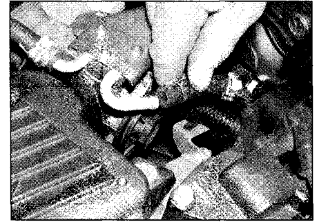
4.6b . . . then disconnect the coolant hoses from the throttle body
