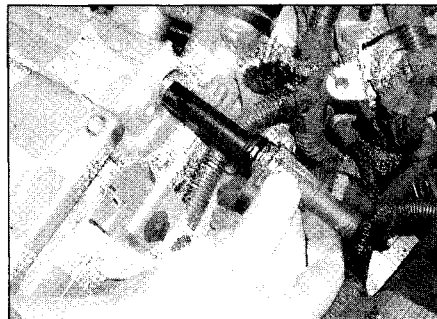
6.2b ... and remove the breather pipe stub
