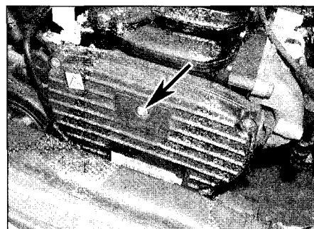
2.4 Remove the screw securing the timing belt upper access cover
