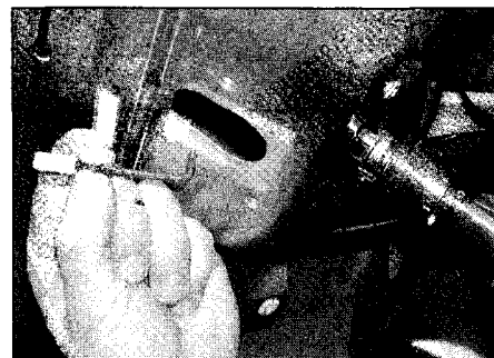
10.7a Disconnect the operating rod ...
