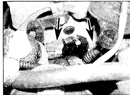
7.4 Ignition power module wiring plugs (arrowed)
