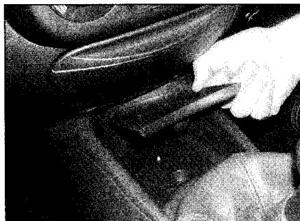
23.4a Remove the covering from the oddments tray in the centre console ...
