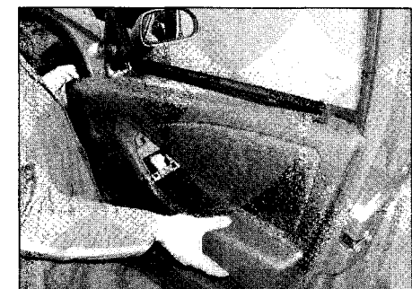
14.5b Lifting the inner trim panel from the door
