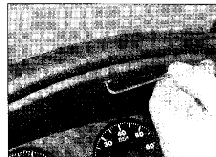
7.6a Unscrew the three upper . . .
