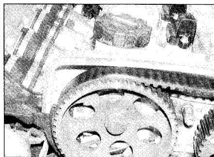
4.11 Mark the camshaft sprockets for TDC position
