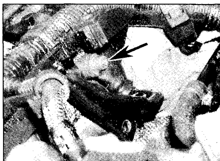
10.4a Unscrew the bolt (arrowed) below the wiring harness bracket . . .
