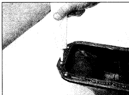
12.4 Applying sealant to the sump flange
