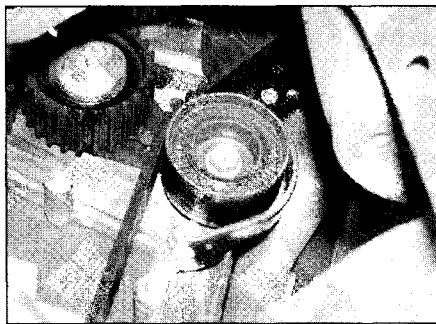
5.29 Timing belt fixed guide pulley
