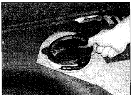
6.3b ... and take off the dust cover for access to the sender unit
