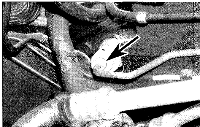
5.8 Union nut on the clutch master cylinder
