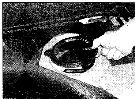
5.3b ... and take off the dust cover for access to the sender unit
