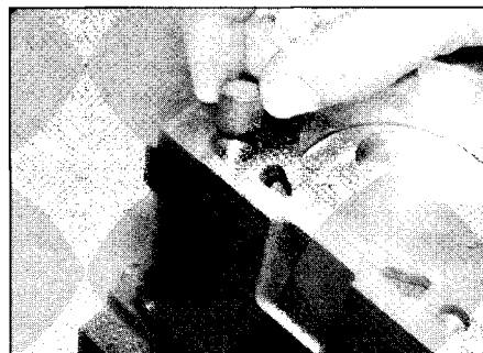
11.29 Refit the cylinder head positioning dowels
