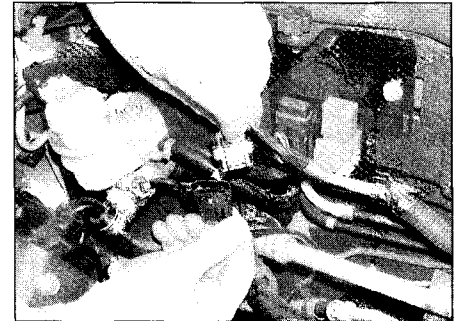
11.11b ... then locate and disconnect the wiring plug for the oxygen sensor
