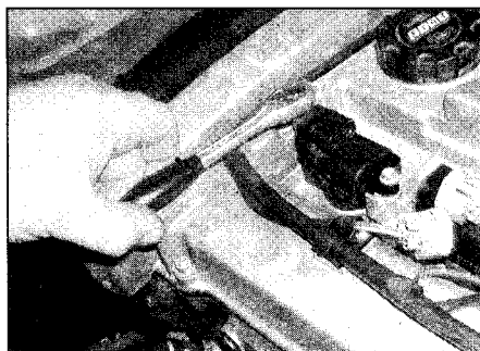
6.7a Unscrew the two mounting bolts . . .
