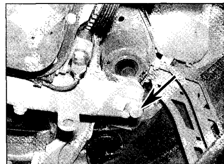
11.7 Engine right-hand mounting (seen from below) - through-bolt arrowed
