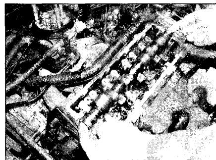
4.10 Lifting out the camshaft on a 1.4 litre engine
