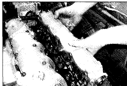
6.14a When removing the housings, tip them over, to prevent the tappets falling out ...
