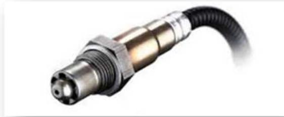
It has one black wire (+ve signal to ECU), one grey wire (signal ground) and two white wires which are for the built in heater element.
