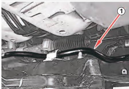
Removing the stabilizer bar
