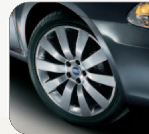
18" alloy wheel kit (Only for versions with ESP) Size 7.5 x 18" (to be fitted in conjunction with 225/45 R18- 95Y tyres). Snow chains cannot be fitted. Part No. 50901442 Kit comprising 4 rims Part No. 50901455 and 4 hub caps Part No. 71801676
