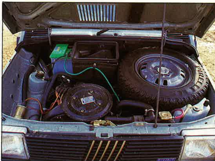
The transverse engine required a unique solution for four-wheel drive
