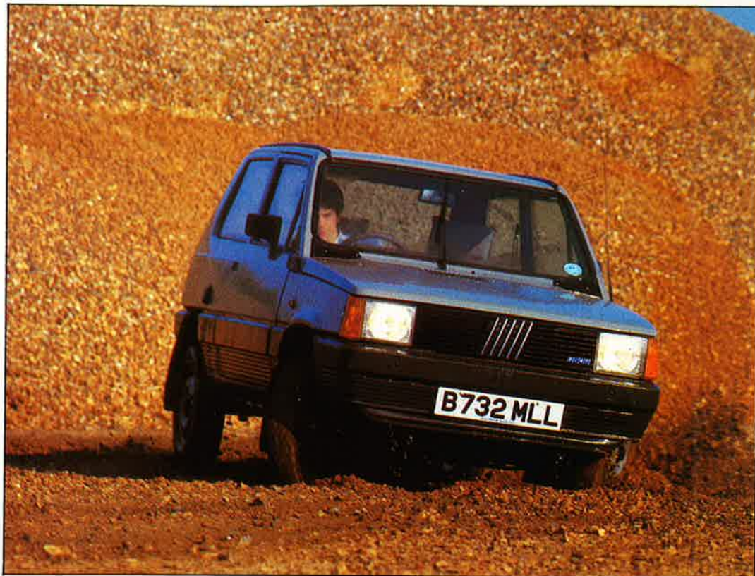
Live rear axle, uprated front suspension and a larger engine make the Panda a good off-roader
