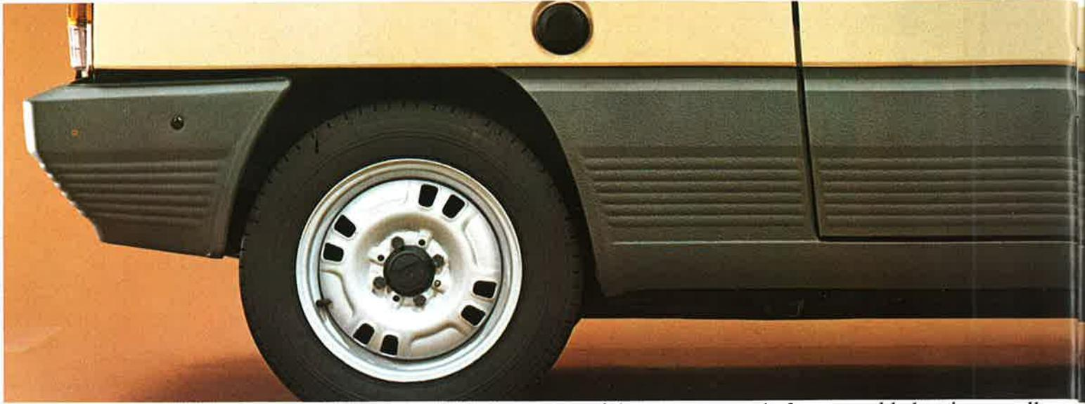
The whole front section of the car as far as the wheel arches is protected by rugged wraparound bumpers
