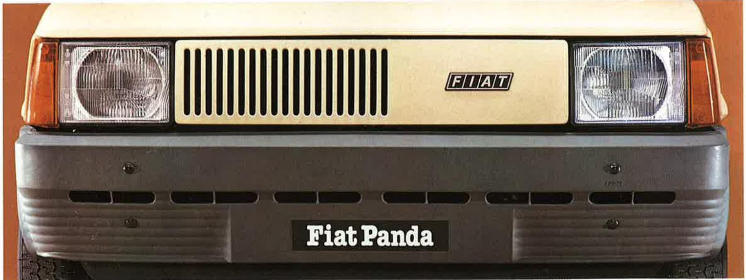
Low-speed impacts can be absorbed by the Panda's bumpers with no damage.
