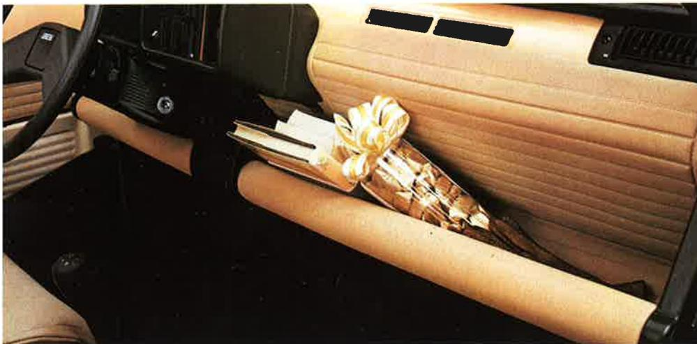
Beneath the dash panel there is a deep full-width and padded oddments shelf in the form of a pouch. The ashtray clips to the tubular edge of the pouch: it is easy to unclip and
