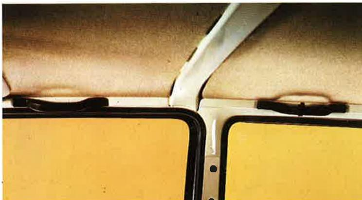
Three grab handles for use by the passengers. A reinforced roll-over bar links the two body sides at door pillar level.
