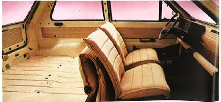
There is also the conventional arrangement which is typical of multi-purpose cars in which the rear seat can either be removed or tilted forward. A luggage compartment capacity of over one cubic metre is thus obtained.
