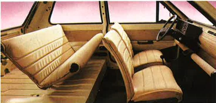
In addition, it is possible to obtain a type of hammock by tilting backward the rear seat and by lifting the leading edge of the cushion. This is extremely useful when it comes to carrying packages, bottles and any other bulky things.
