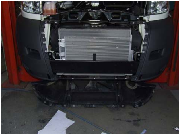
Figure 1 - Under body guard dropped away from vehicle
