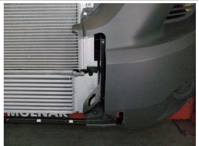
Figure 4 – Completed trim section from front of side bumper sections..
