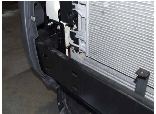
Figure 2 – Bumper support, drivers side shown
