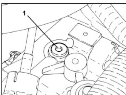
1. Remove the automatic transmission fluid filler plug.
