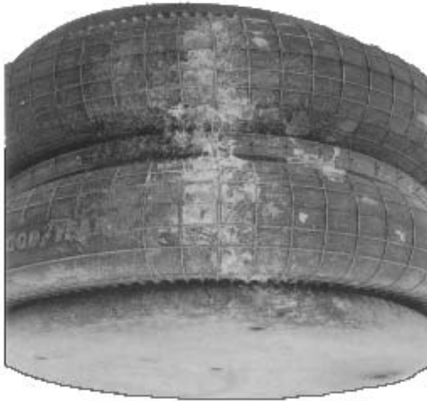
Deterioration of the bellow - is caused by chemicals that, in time, literally eat a hole in the rubber.
