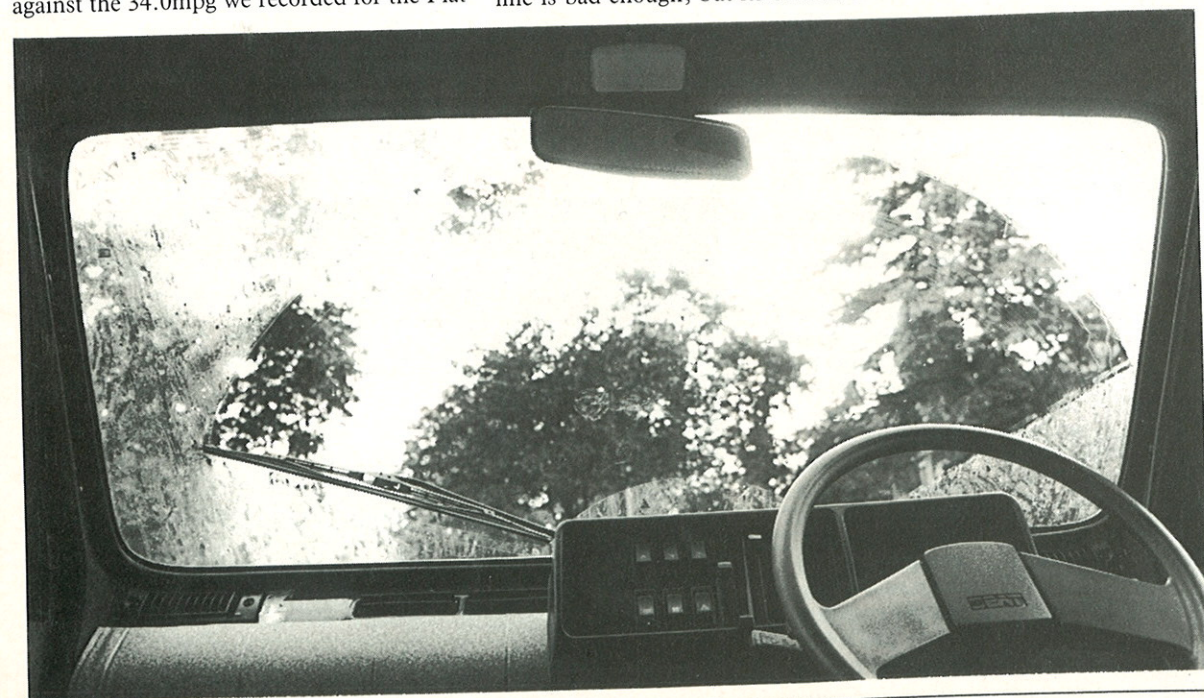
The single windscreen wiper is inadequate, leaving large areas of the screen untouched
