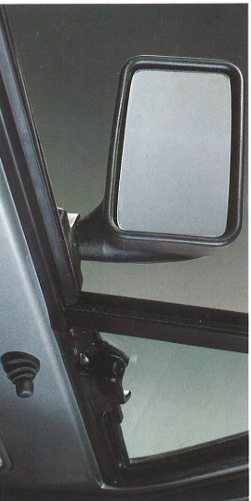
Door mirror adjustable from inside.
