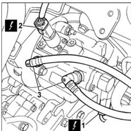
1. Disconnect the electrical connection for the fuel pressure regulator.
