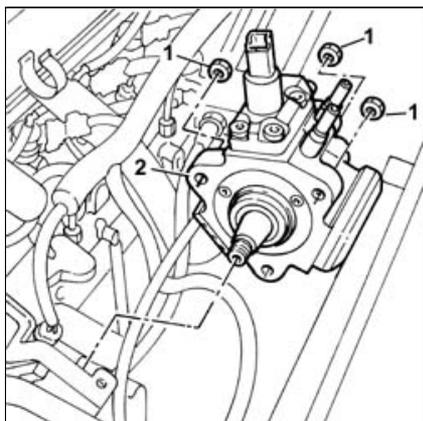
1. Undo the fixing nuts.
