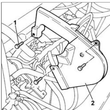
1. Undo the fixing bolts.
