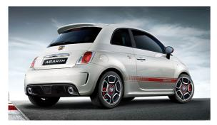
The 500 Abarth optimises aerodynamic behaviour with several elements, including a large winged spoiler and a 'diffuser' that links up to the underbody, optimising the airflow output, and involving much of the rear bumper. We should underline that these latter two elements – the spoiler and the diffuser – help to reduce drag and increase downforce at high speed.
