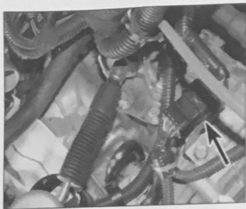
4.12a Disconnect the main wiring harness connector (arrowed) at the top of the transmission . . .
