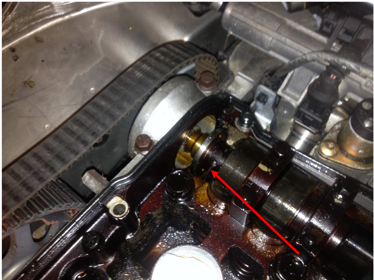
Picture 1 – showing the black circlip that holds together the outer part of the variator with the camshaft.
