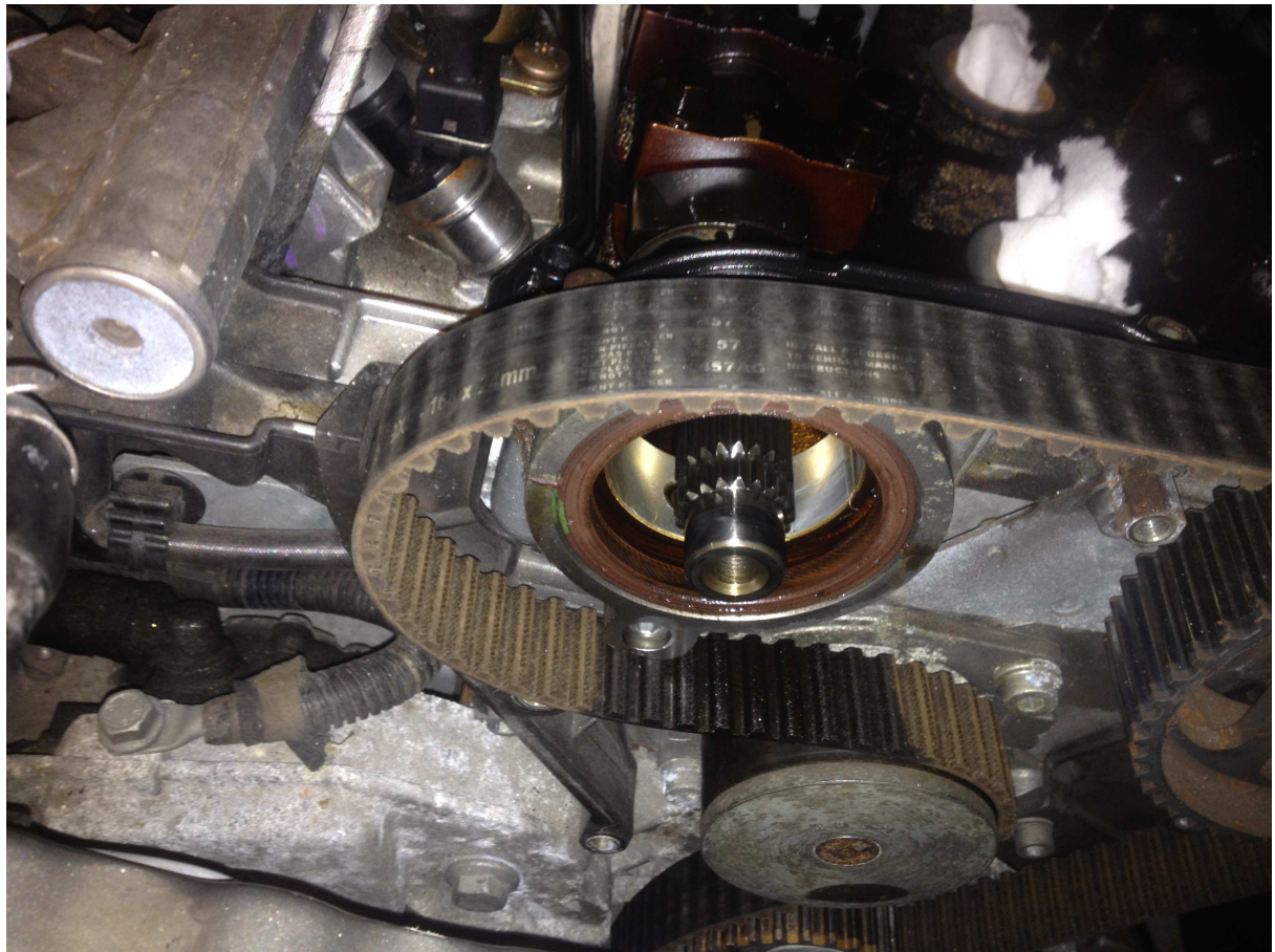
Picture 2 – the spines on the shaft where the variator sits.
