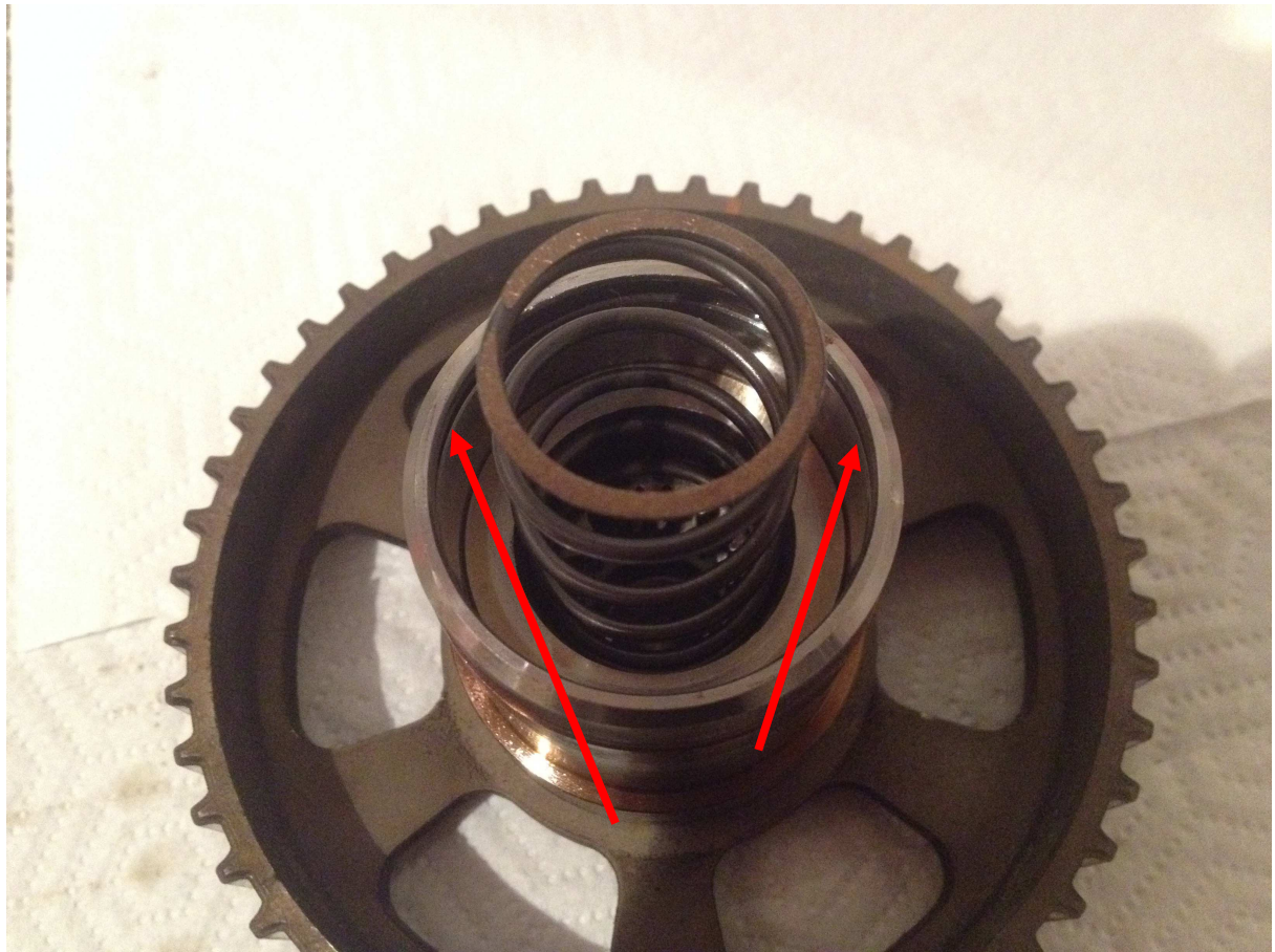
Picture 4 – This is the groove where the black circlip engage, to keep the variator on the camshaft. Make sure this is clean to make room for the circlip to fully expand when putting back the variator.
