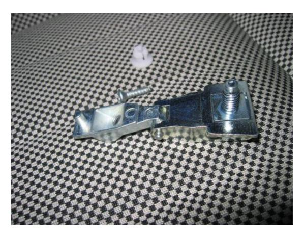
The pozidrive screw retaining the other part of the broken hinge in the door handle can be undone through the hole in the door!
