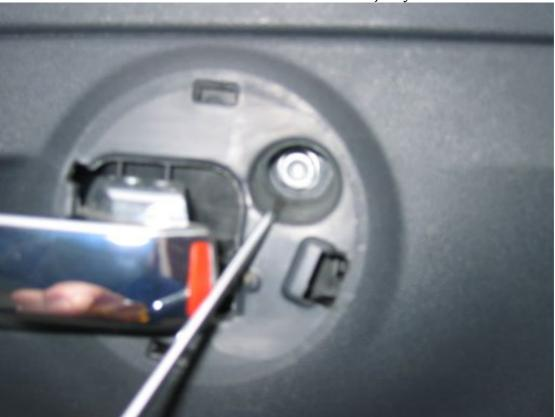
Now start to ease out the plastic plugs which hold the door card to the inner door frame by starting in the bottom corner furthest from the door hinges.....this can
