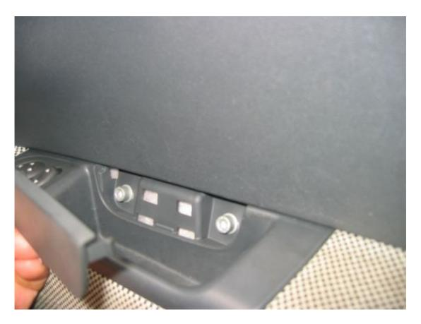
Next I prised off the chrome (plastic, so be gentle) bezel around the inner door handle by easing a small screwdriver in at the front (door hinge) end...
