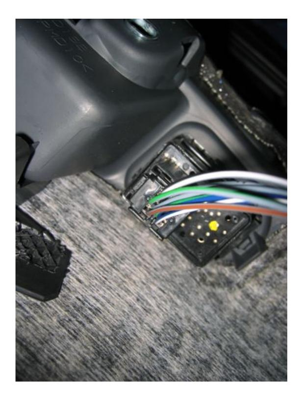
OR (as I did) by removing the mirror switches panel, lifting it up and out by pressing the release lug (indicated by the screwdiver) and then removing the (then) more accessible wiring plug....
