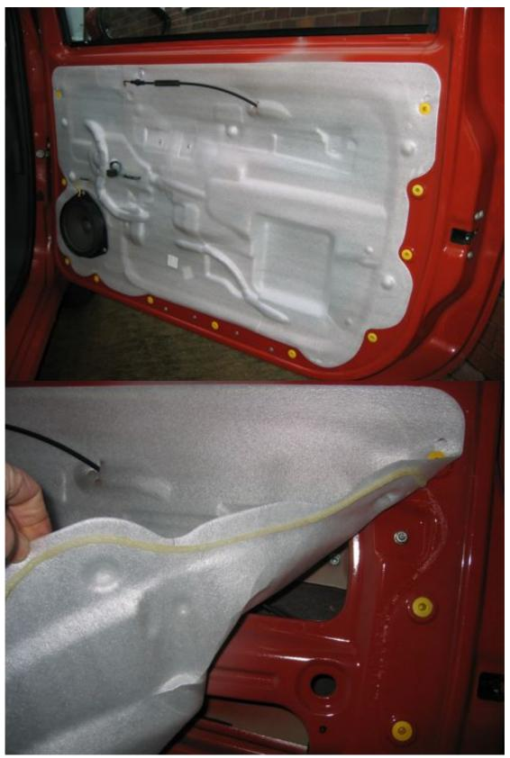
You can just see inside the door the 10mm nut at the back of the handle's broken hinge. Remove the nut and discard the broken hinge, but keep the nut; you don't get another.
