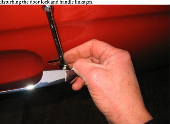
Swing the hinge round to its closed position and its threaded bolt can then be slotted through the hole and the 10mm nut tightened on it
