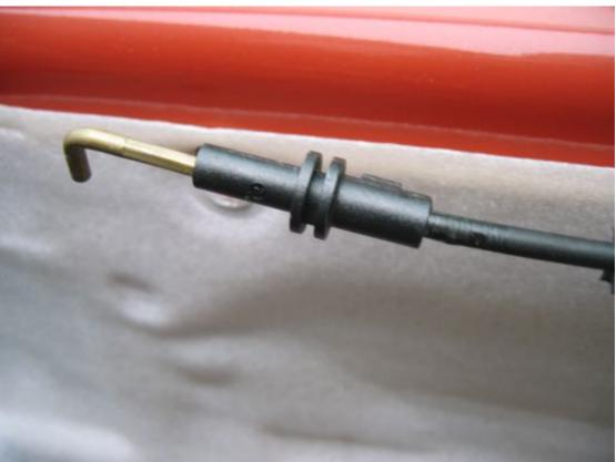
And now start to lift up the polystyrene door skin very carefully using the blunt flat bladed screwdriver.....this is what takes the time if you want it to go back intact and using the same glue......it worked for me, and simply pressed down and held tight when I was putting it all back together.
