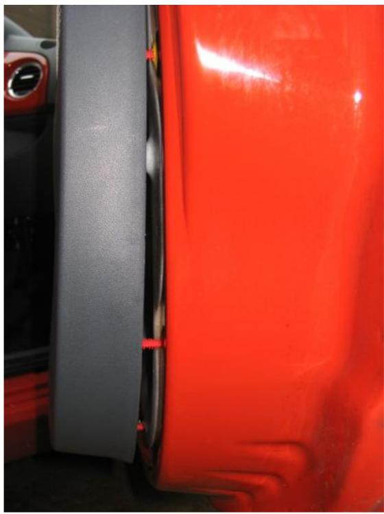
The next photograph shows where all the red plugs are positioned and once they are all 'popped out", the 3 allen bolts can be removed, and the door card unhooked from the top where it lips over the door window ledge, but it still can't be removed more than about 6 inches from the door as it is still attached to the wiring loom and to the door handle cable.
