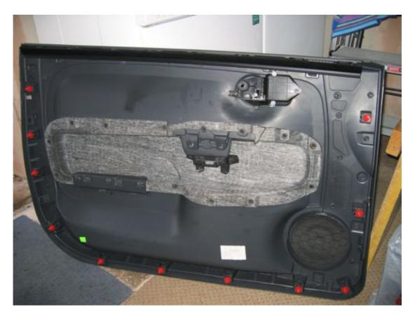
So now to remove the wiring loom link by EITHER pulling out the plug by pressing a release tab on its rearward side (near to the green wire in the photo)
