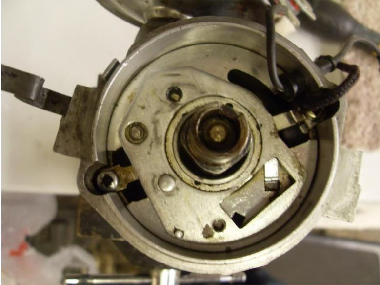
Below the contact breaker base plate is the actual Advance/Retard mechanism.
