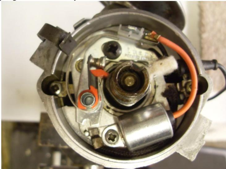
The points are fixed to a base plate and some small adjustment is possible via the black pozi screw to enable the correct gap to be set.
