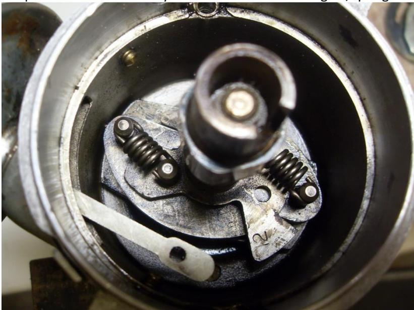
As the dizzy spins and the weights fly out due to centrifugal force they move the cam lobe in the opposite direction to the dizzy rotation which has the effect of advancing the timing.
