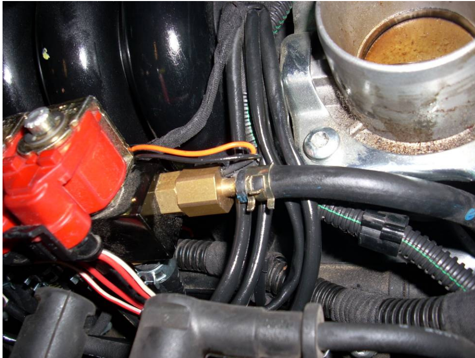
Temperature sensor connection
