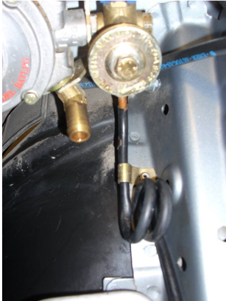
Tube connection to inlet of solenoid valve
