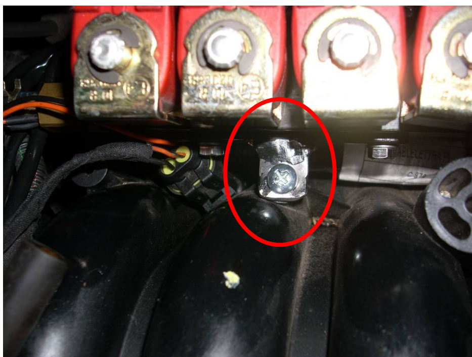
Injector rail hard support
