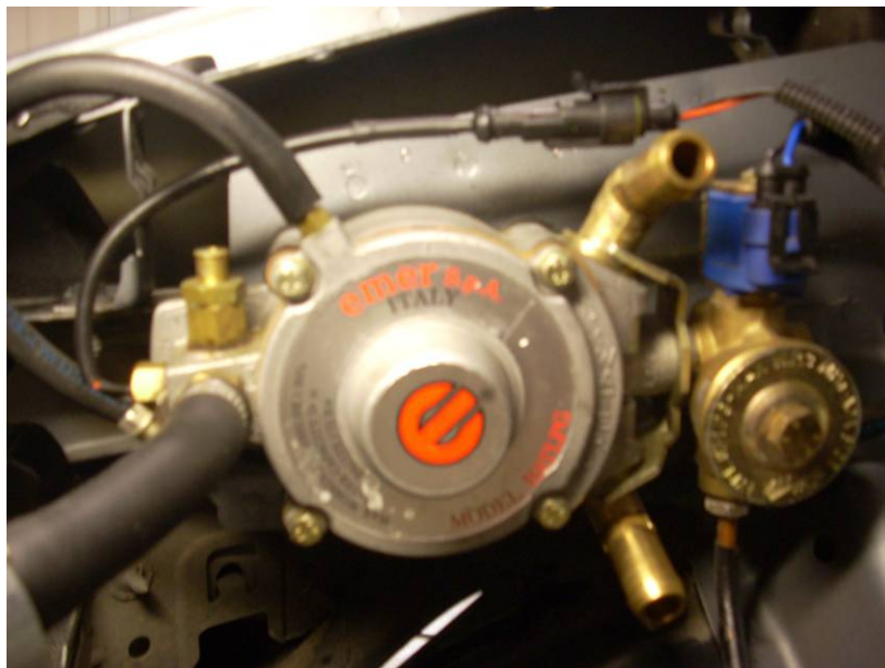
Pressure reducer with solenoid valve
