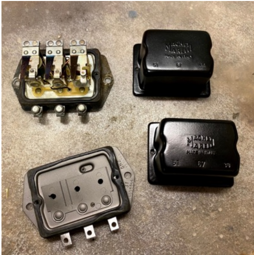
Original-style voltage regulator (top) and modified voltage regulator (bottom)
