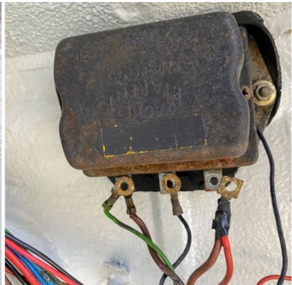
Modified voltage regulator ( left ) installed. Here you can see where I used the old mounting posts as ‘cosmetic’ junctions.
