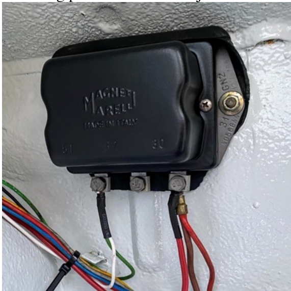
Modified voltage regulator ( left ) installed. Here you can see where I used the old mounting posts as ‘cosmetic’ junctions.
